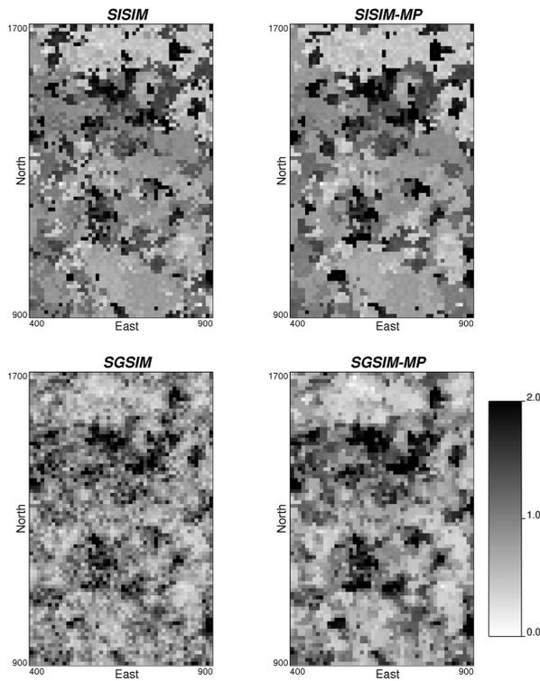
**Figure 2.** Plan views of the two benches simulated using sequential indicator simulation updated with multiple-point statistics.
